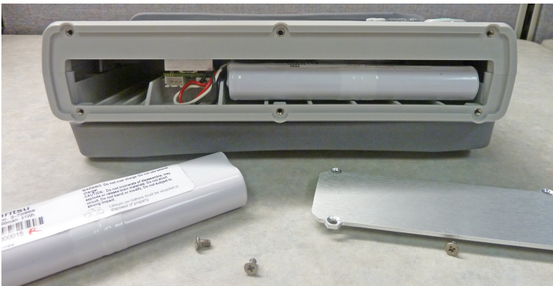
Figure 10-3. Replacing the Batteries
