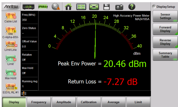
Figure 6-6. Power Meter View
